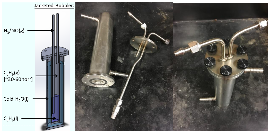
FIG. 5. Left: SolidWorks jacketed high pressure bubbler. Right: Photos of a jacketed high pressure bubbler.
