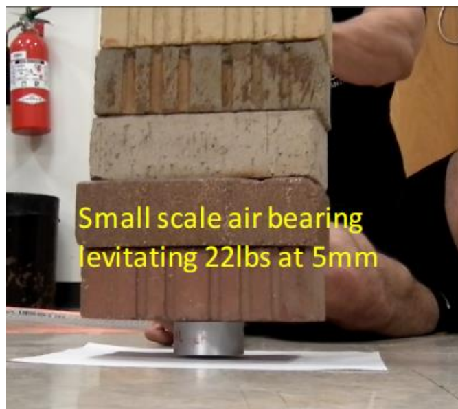
Figure 2.3. A small-scaled prototype of an air bearing as designed by the TAMU Hyperloop team. Reprinted from Texas A&M Hyperloop with permission from TAMU Hyperloop (Karpetis, 2017). [18]
