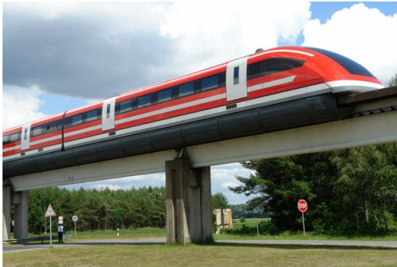
Figure 3.2. Maglev train systems are known to travel at high speeds with the use of a magnetic suspension system. Reprinted from Maglev (Wikimedia, Public Domain, 2018). [45]
