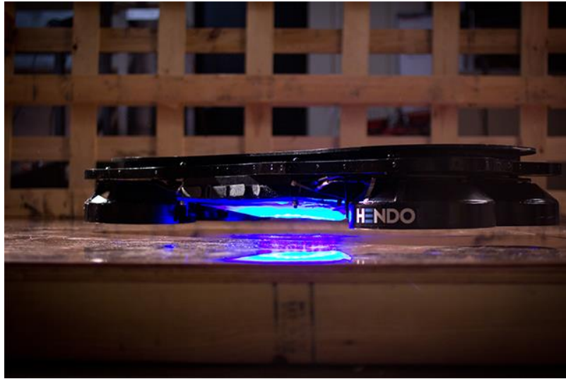
Figure 7.1. The Hendo board from Arx-Pax uses active maglev technology for levitation applications. Reprinted from Hendo Hover (Kickstarter, 2014). [13]
