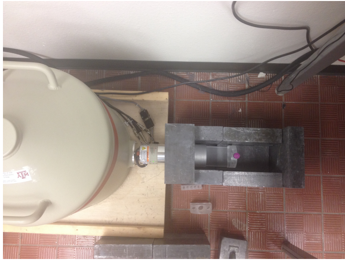
Figure 2.13: HPGe detector system with geometry and dewar shown.
