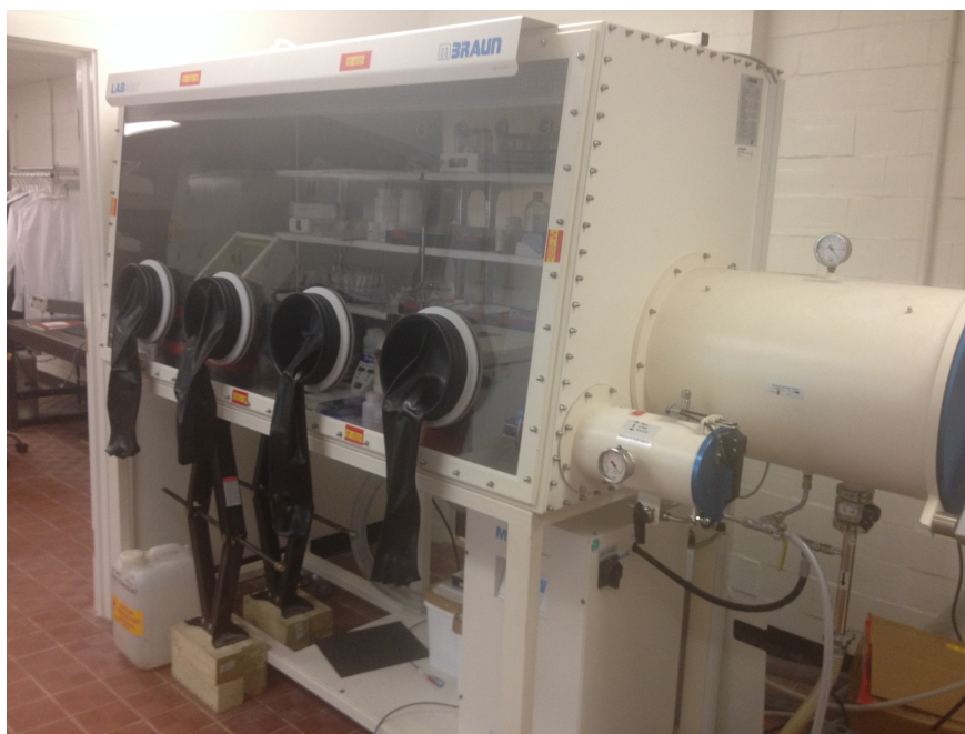
Figure 2.9: Glove box workstation.
