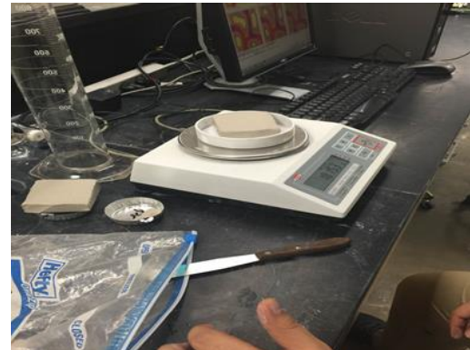
(d) weighing the soil to check when equilibrium had been reached
