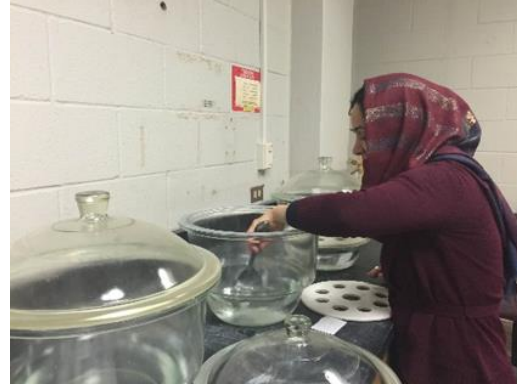
(c) mixing predefined amounts (g) of water and salt to have solutions with exact salt concentrations
