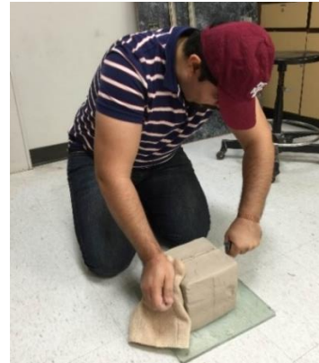
(b) cutting a soil block
