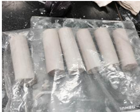
(e) protecting samples from moisture loss in a properly sealed, air-tight container
