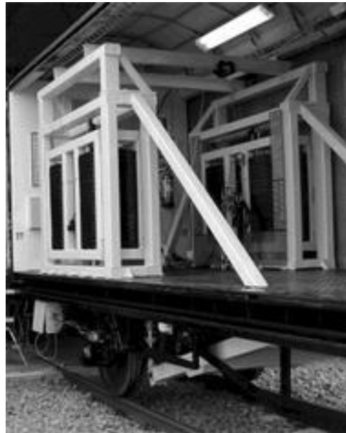
(a) The KTH rolling stiffness measurement vehicle
