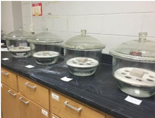
(c) put the soil sample inside the closed chamber and wait for equilibrium
