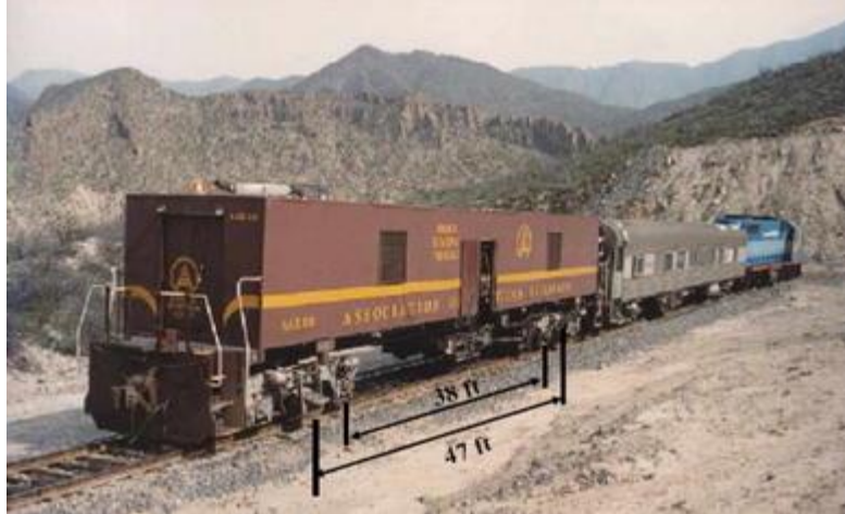
(a) The track load vehicle developed by the Transportation Technology Center, Inc. (Nicks 2009)
