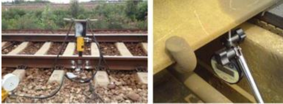
(a) Jack-loading diagram and vertical rail displacement measurement (Wang et al. 2016)
