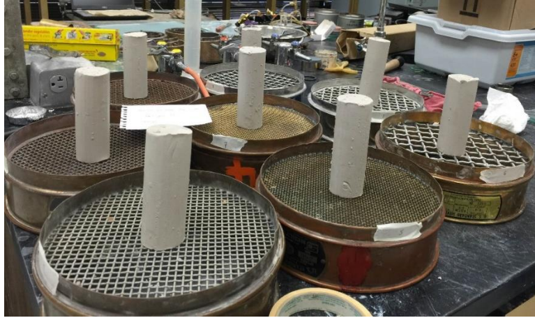
Figure 3.16. Six samples on top of the sieves to air dry uniformly
