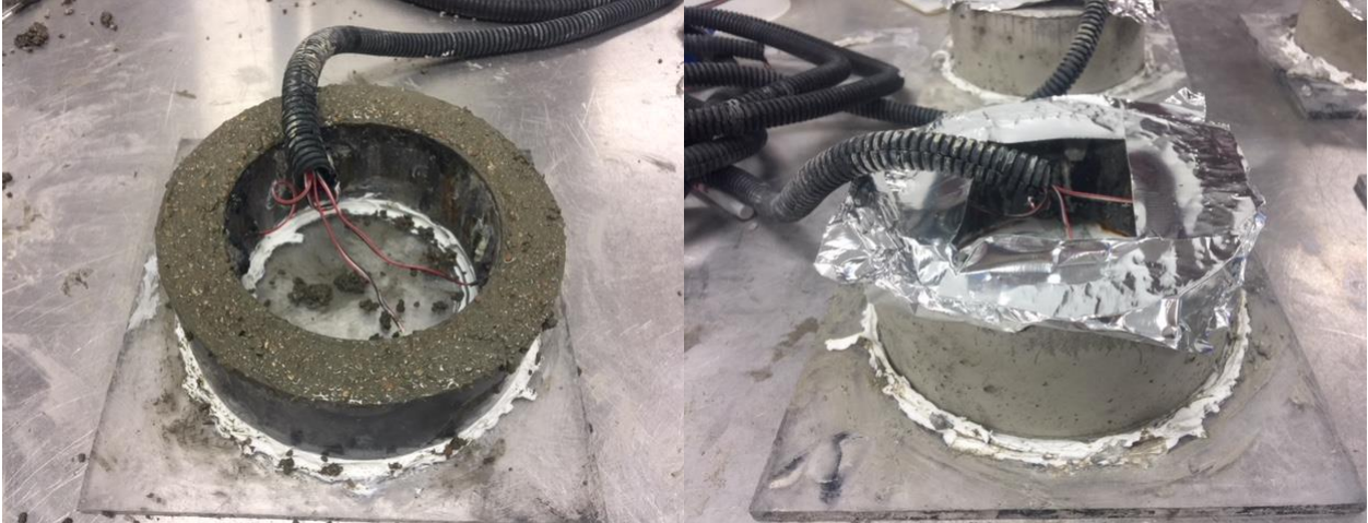
Figure 30 Mortar ring test: a mortar ring after casting (left) and at the end of the testing period (right)
