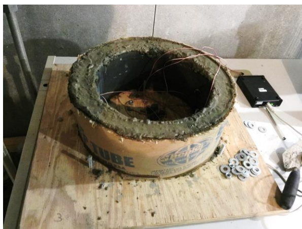
Figure 29 Ring Test: concrete ring at age of 1 days (left) and at age of 28 days
