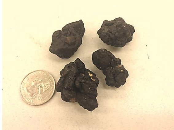
Figure 21 Agglomerated particles in AMA
