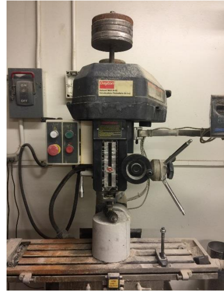
(b) Rotating cutter approach, ASTM C944
