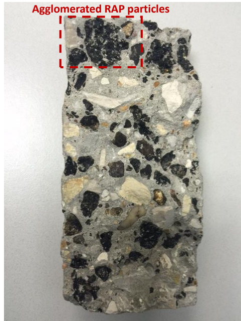
Figure 46 Agglomerated RAP particles from a cross section view of the 0.40_520_40AMA
