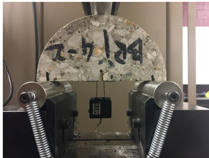
Figure 36 SCB fracture test set-up
