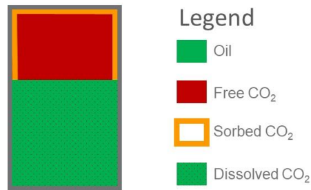
Figure 70 – Schematic representation of the three components of CO 2 storage. Free CO 2 in the porous space, sorbed CO 2 in and on the organic matter and dissolved CO 2 in the remaining oil.
