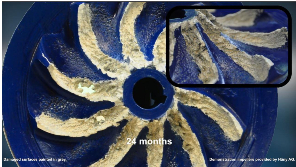
Figure 5: Pump impeller with damage from 24 months of cavitation damage. [8]
