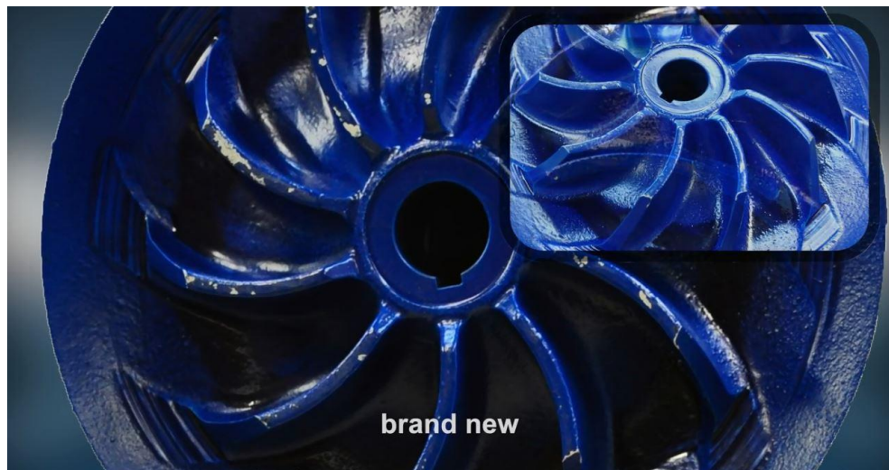
Figure 4: Pump impeller with no cavitation damage. [8]
