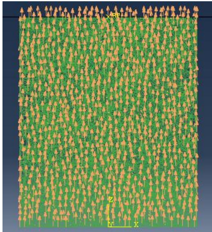
Figure 25. Boundary conditions for impact analysis of specimen with 82,335 beam elements and changing porosity
