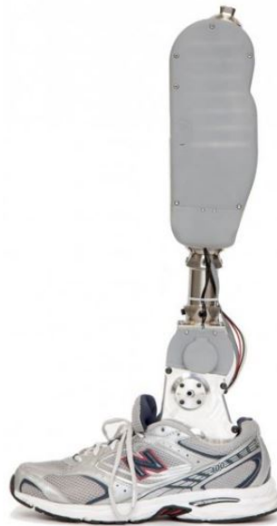
Figure 1.4: Center of Intelligent Mechatronics at Vanderbilt University, the powered prosthetic system designed to provide the net power for the ankle and knee joints [4]
