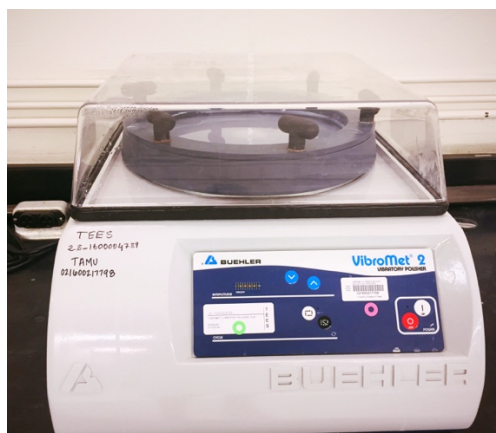
Figure 2.12 VibroMet 2 vibratory polisher to prepare high quality polished surfaces.
