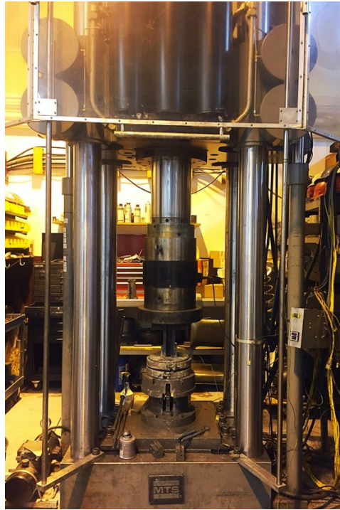
Figure 2.5 Equal channel angular extrusion die to provide severe plastic deformation.
