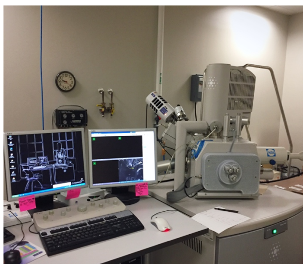
Figure 2.13 FEI Quanta 600 FE-SEM used for high-resolution imaging of surfaces.
