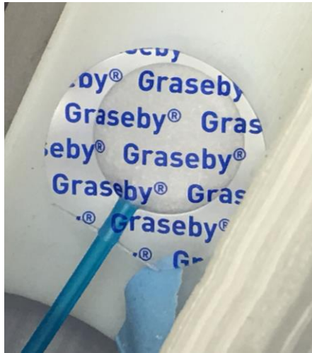
Figure 17. This figure portrays the BIOPAC respiratory gating detector. This detector will allow monitoring of the mouse breathing and how much aerosol is being delivered based on the breathing pattern.
