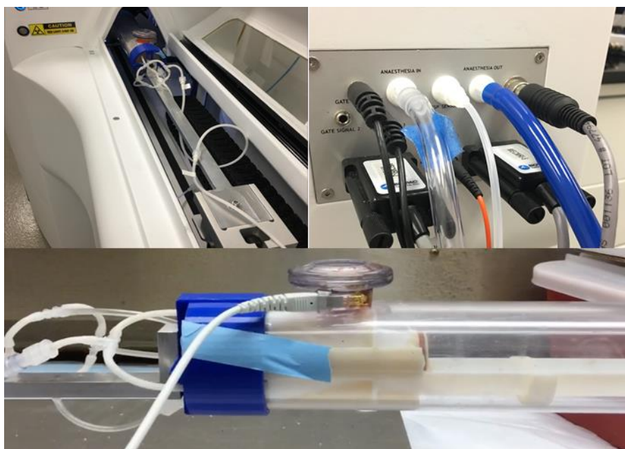
Figure 15. The assembly of the device with vacuum and anesthesia lines connected in the rear and the AeroGen nebulizer mounted on top and integrated into the Albira Si.
