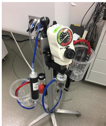
Figure 16. The vacuum system used during experimentation. This vacuum system would remove any potential leakage of fluorescent probe or radionuclide from the mouse housing portion of the nebulizer system.
