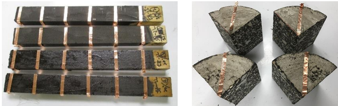
(a) Mastic specimens with various graphite contents for determining electrical characteristics
