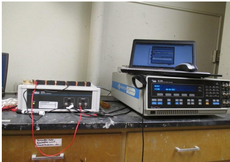
(b) Resistivity measurement set-up: Solartron 1296 & 1260A
