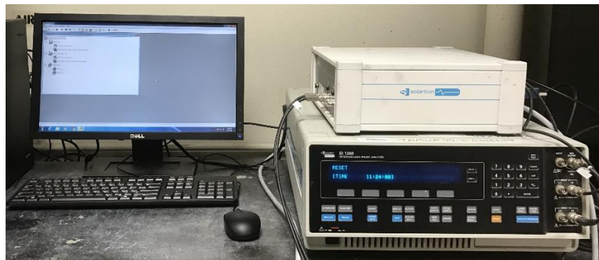
Figure 28. Resistivity measurement set-up: Phase gain/phase analyzer (Solartron 1296 & 1260A)
