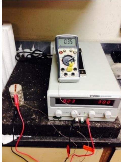
Figure 59. Experimental set-up for measuring electrical heating (DC)
