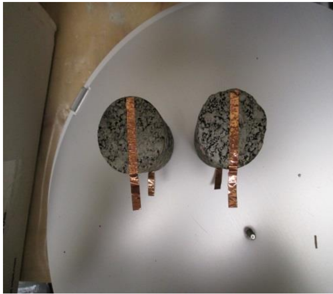
(b) Installing copper tapes as electrodes
