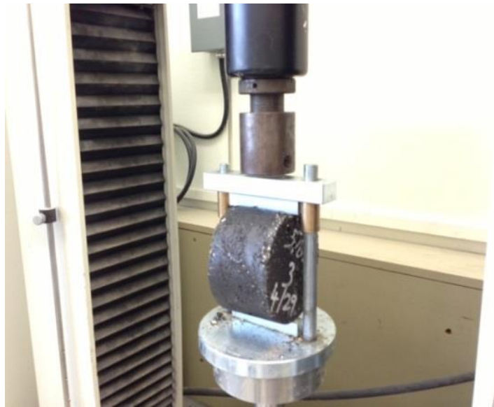
Figure 16. Indirect tension test set-up
