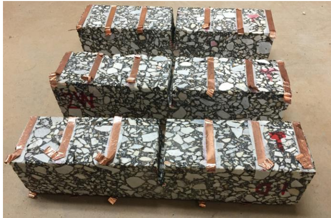
(a) Asphalt concrete samples for damage sensing
