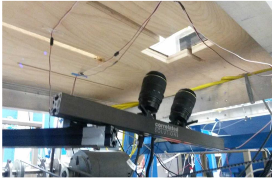
On the left: lenses setup under the wind tunnel section. Lenses aim at a Plexiglas panel installed on the floor of the wind tunnel.
