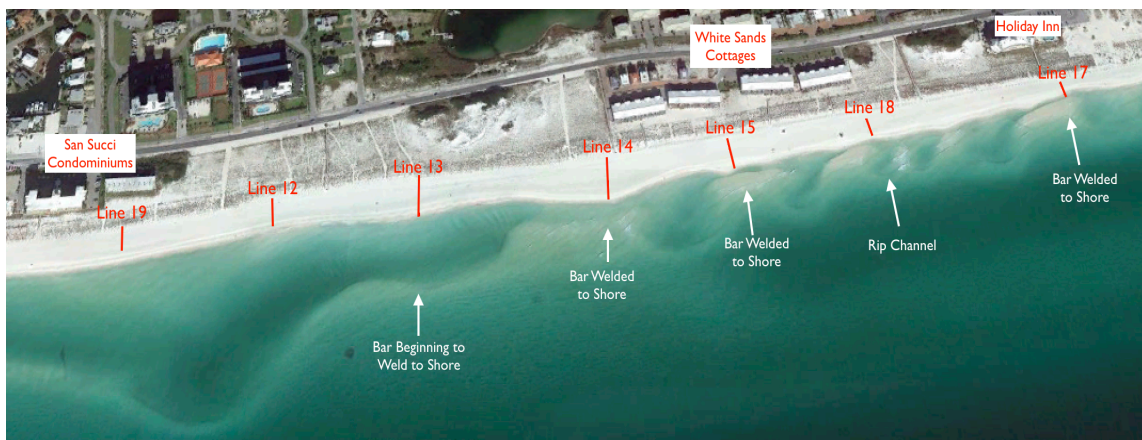
Figure 40: Locations of 500 MHz crossshore GPR lines. The areas where the bar welded to shore are labeled as well as the rip channel.
