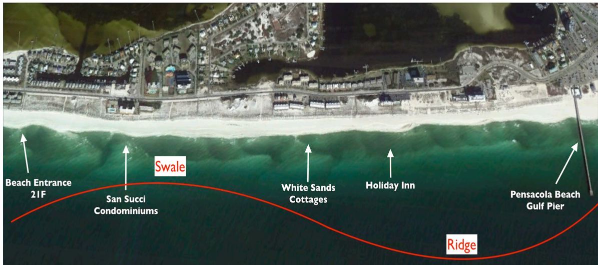
Figure 37: Ridge and swale topography is typical of Santa Rosa Island. In the study area, there is a swale centered on the San Succi Condominiums and two ridges; one ridge at Fort Pickens Gate (east of beach entrance 21F) and the other ridge is centered on the Pensacola Beach Gulf Pier. (Location of ridge and swale from Houser, 2012)
