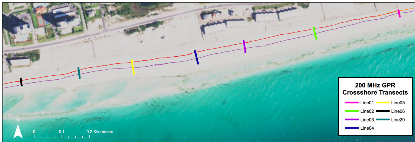
Figure 8: Map showing the path of the 200 MHz alongshore GPR transects with corresponding 200 MHz cross-shore transects.
