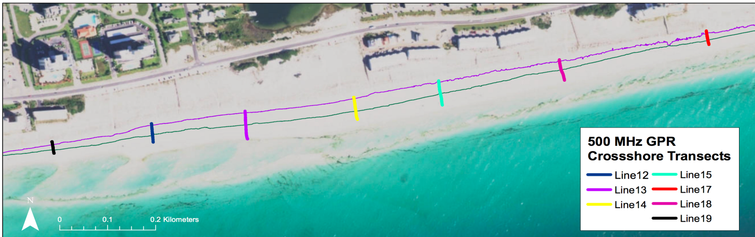
Figure 10: Map showing the path of the 500 MHz alongshore GPR transects with corresponding 500 MHz cross-shore transects.
