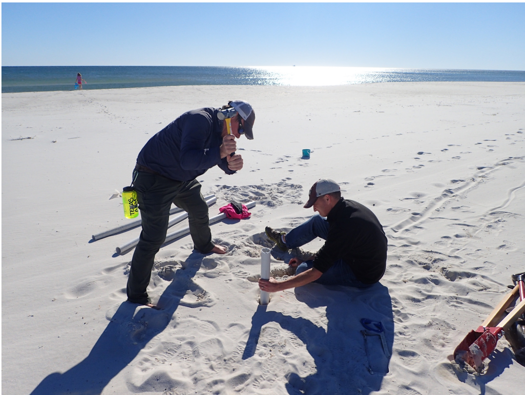
Figure 11: Modified Coring system created using 3- inch diameter PVC pipe and Sledge hammer.
