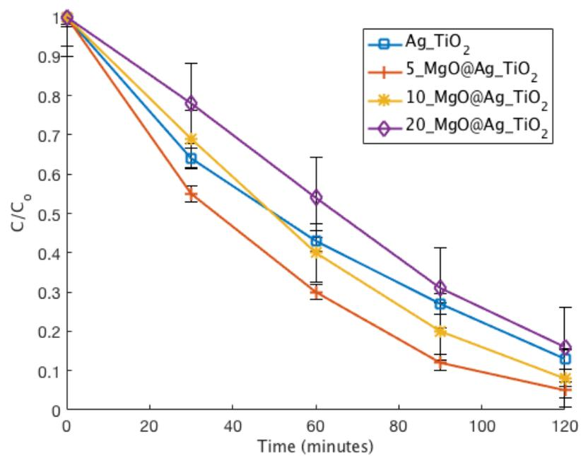
**Figure A2: Effect of number of MgO cycles on phenol degradation for varying irradiation times**
