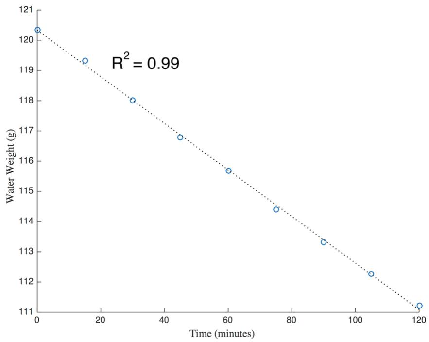
**Figure A7: Water evaporation rate by cooling fan**
