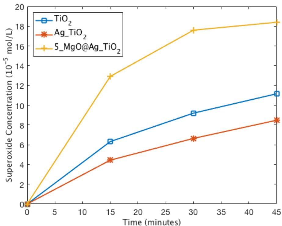
**Figure 10: Superoxide production for TiO<sub>2</sub>, Ag\_TiO<sub>2</sub>, and 5\_MgO@Ag\_TiO<sub>2</sub>**
