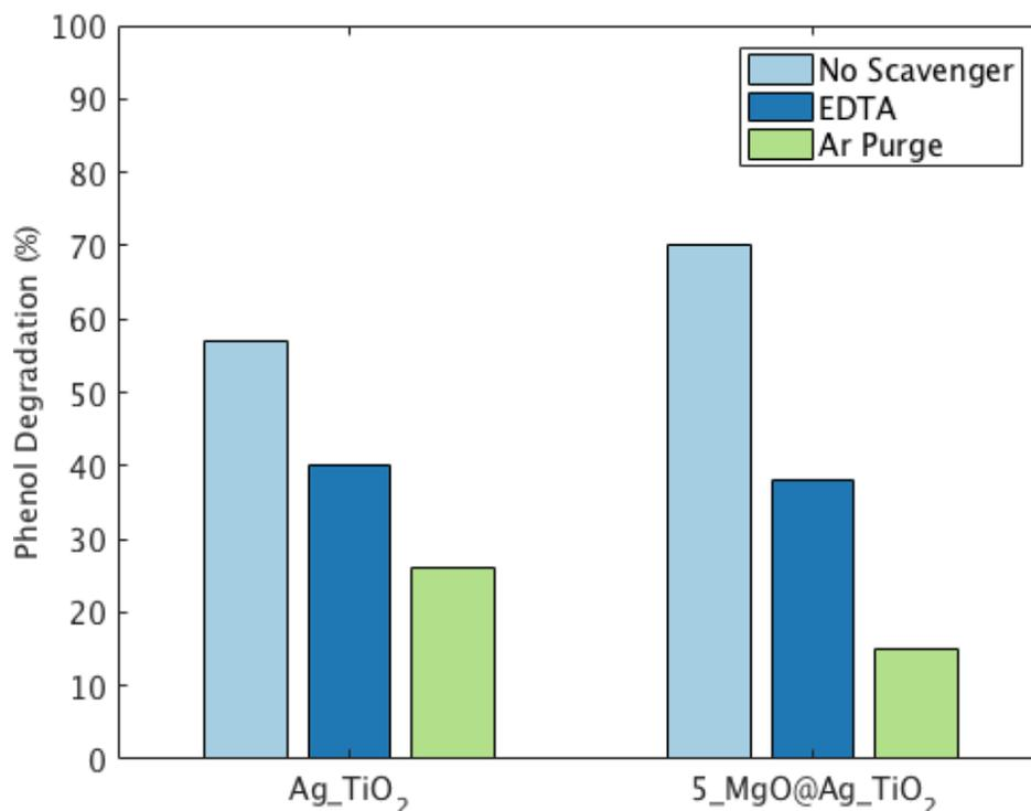
**Figure 8: 60 min scavenger study results for Ag\_TiO<sub>2</sub> and 5\_MgO@Ag\_TiO<sub>2</sub>**
