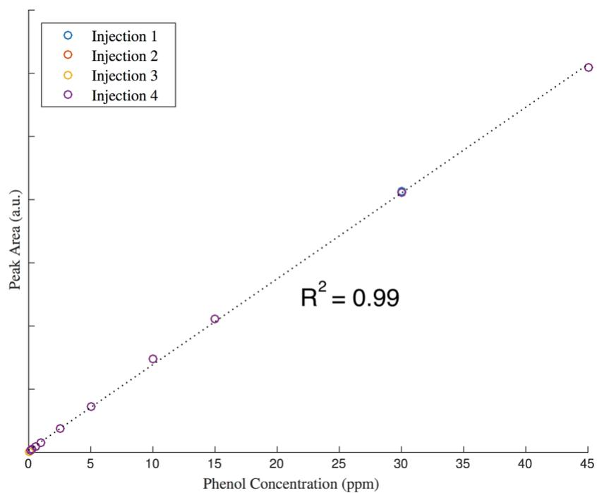
**Figure A5: HPLC phenol calibration from 0.015-45 ppm, four separate injections per concentration level**
