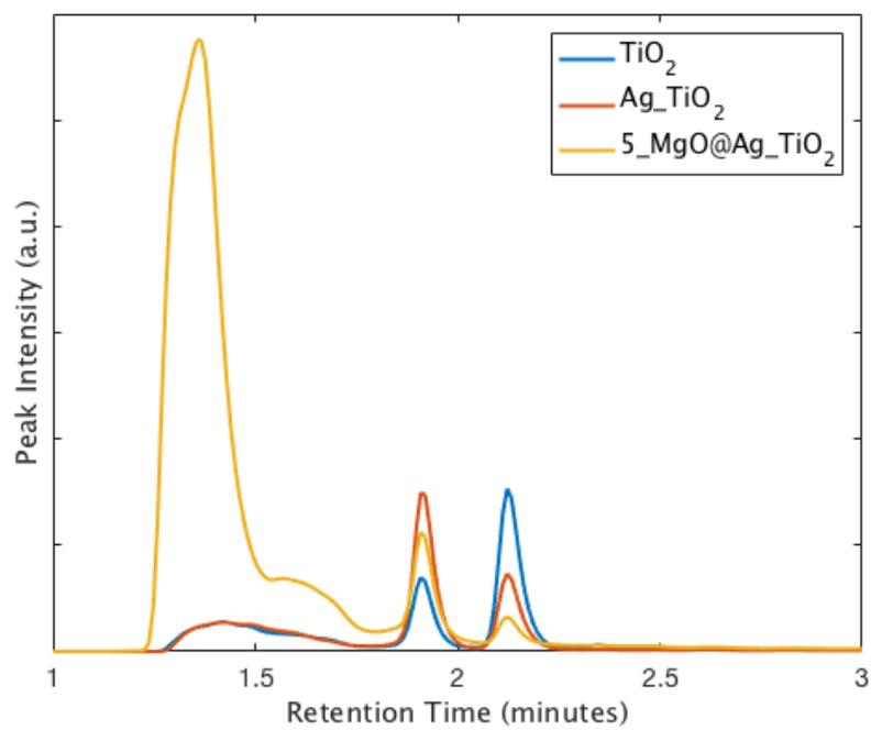
**Figure A4: HPLC Spectra for  $\text{TiO}_2$ ,  $\text{Ag-TiO}_2$ , and  $5\text{-MgO@Ag-TiO}_2$  after 120 minutes irradiation**
