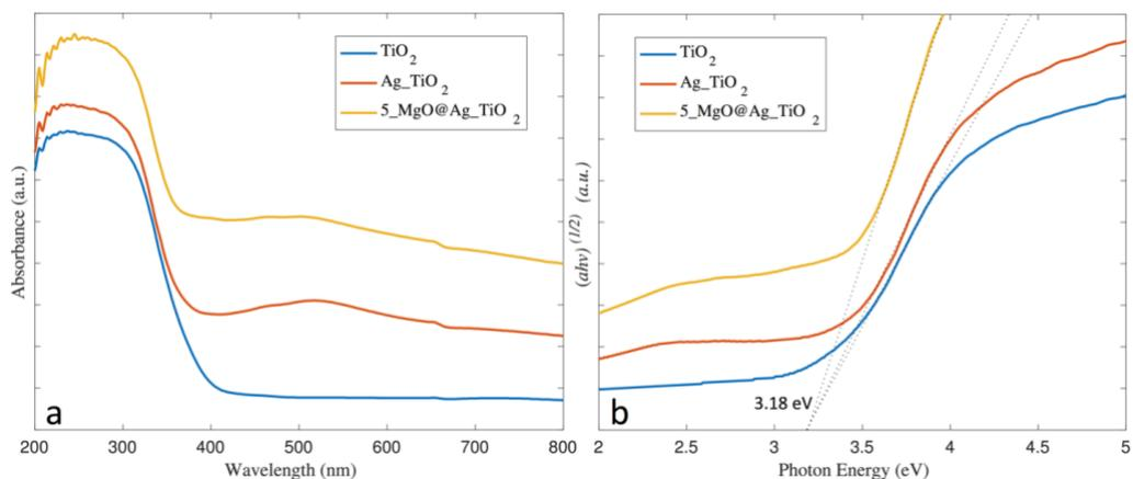
**Figure 4: (a) UV-Vis Diffuse-reflectance spectra and (b) Tauc plot for  $\text{TiO}_2$ ,  $\text{Ag-TiO}_2$ , and  $5\_MgO@Ag-TiO_2$**
