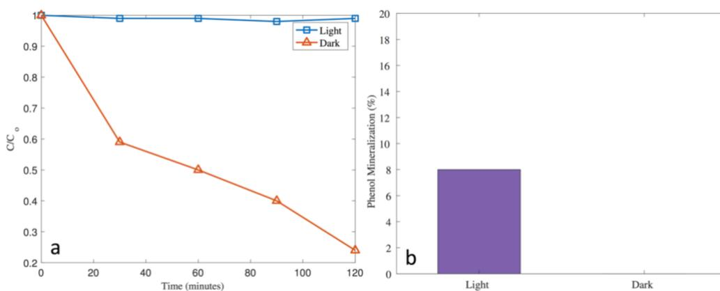
**Figure 11: Phenol 120 min (a) degradation and (b) mineralization by the addition of 0.3mM  $\text{H}_2\text{O}_2$**
