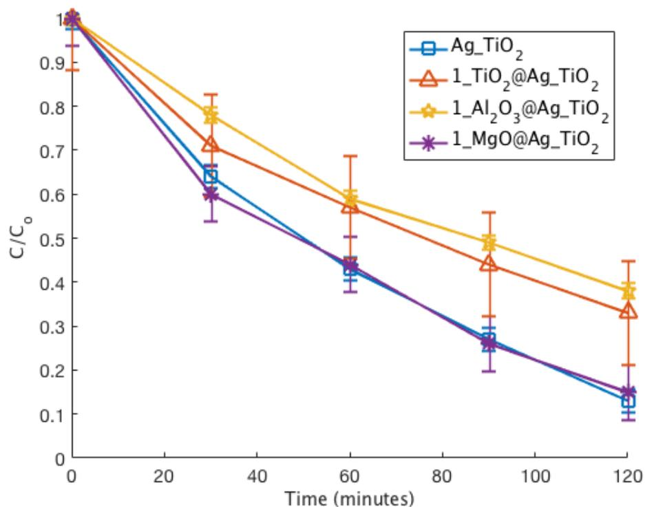
**Figure 5: Effect of metal oxide coating material on 120 min degradation of 50 ml 15 ppm phenol solution with 0.2 g/L catalyst loading under solar irradiation**
