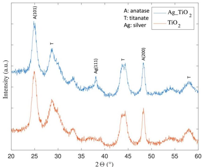
**Figure 3: XRD Spectrum of  $\text{TiO}_2$  and  $\text{Ag}_x\text{TiO}_2$**
