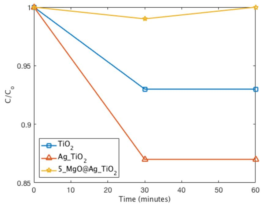
**Figure A3: Adsorption equilibrium of phenol for  $\text{TiO}_2$ ,  $\text{Ag-TiO}_2$ , and  $5\text{-MgO@Ag-TiO}_2$**
