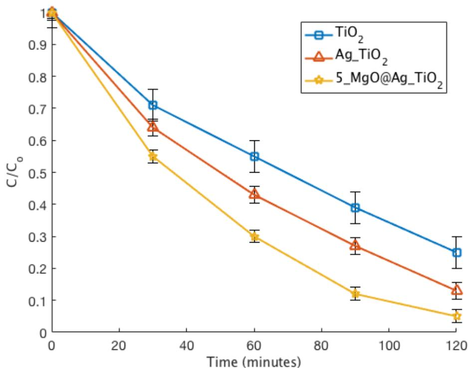
**Figure 6:  $TiO_2$ ,  $Ag\_TiO_2$ , and  $5\_MgO@Ag\_TiO_2$  120 min degradation of 50 ml 15 ppm phenol solution**
