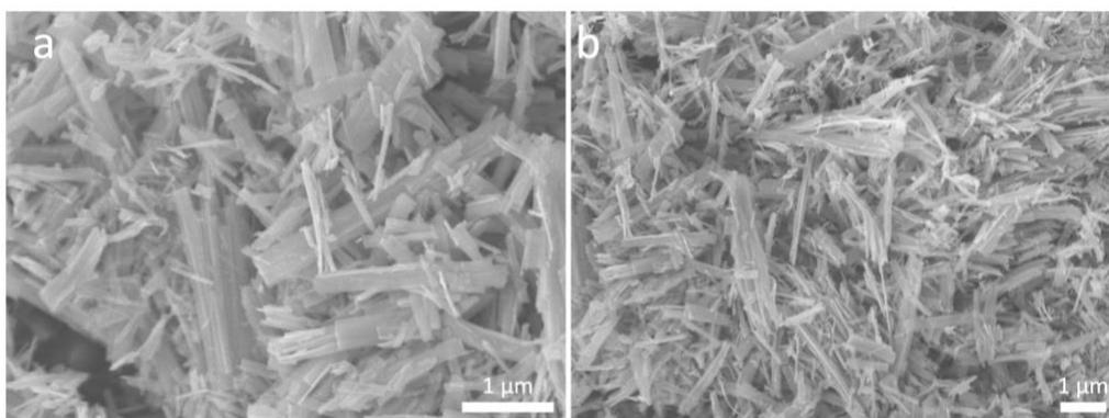
**Figure 2: Geometry of synthesized  $\text{TiO}_2$  nanorods**
