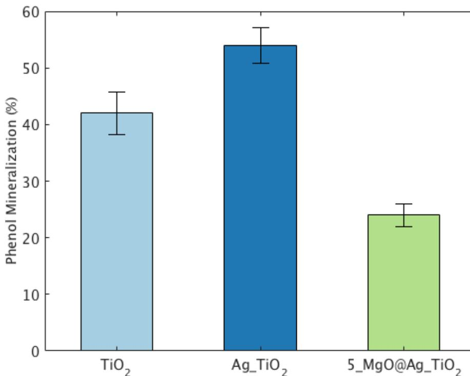
**Figure 7: Phenol mineralization by TiO<sub>2</sub>, Ag\_TiO<sub>2</sub>, and 5\_MgO@Ag\_TiO<sub>2</sub> of 50 ml 15 ppm phenol solution with 0.2 g/L catalyst loading after 120 min solar irradiation**
