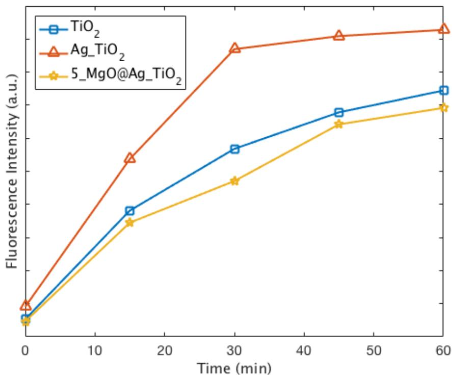
**Figure 9: HTA fluorescence for TiO<sub>2</sub>, Ag\_TiO<sub>2</sub>, and 5\_MgO@Ag\_TiO<sub>2</sub>**
