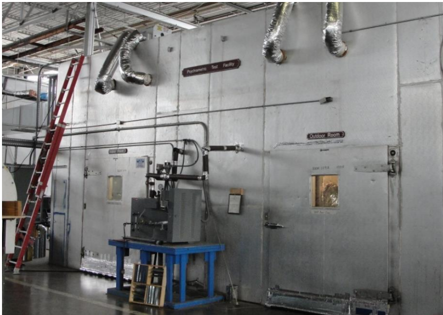
Figure 5: Psychrometric test chamber at REEL facility.
