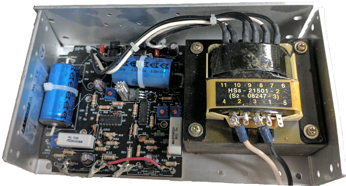
Figure 3.20: One of the three power supplies from TDK-Lambda used to power the motor.
