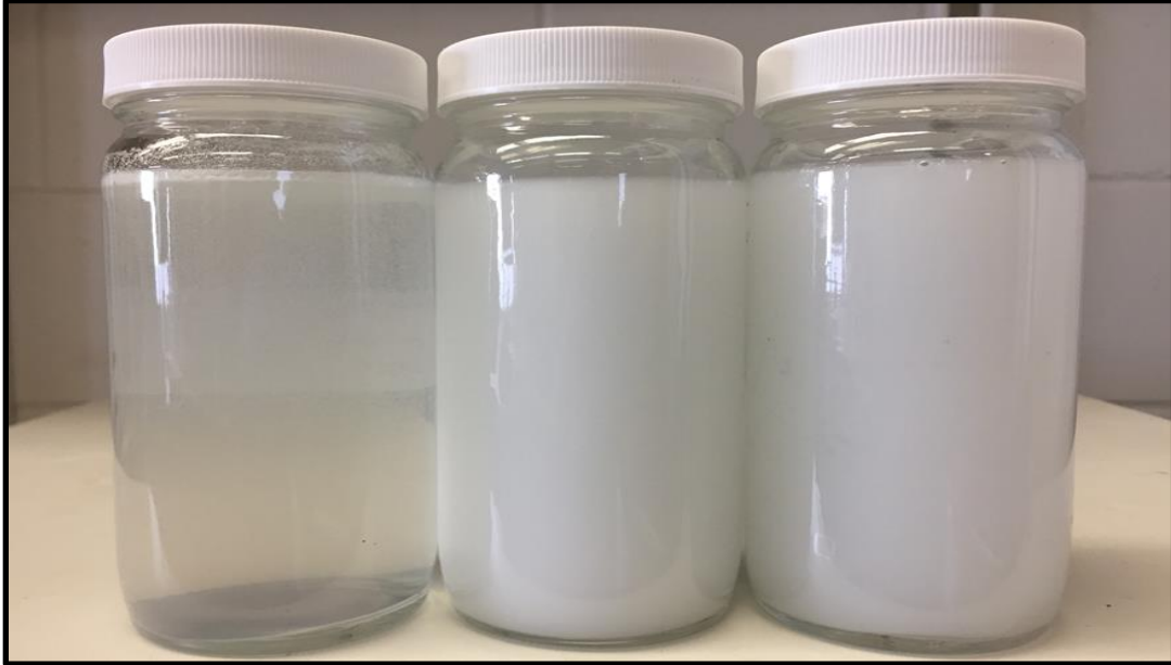
Fig. 36 – (Left) 40 lb/1,000 gal CMHPG, (Middle) 1:1 (CMHPG: Synthetic) polymer mix, (Right) Synthetic polymer, mixed with 10 ppt sodium bromate and 4 gpt crosslinker at pH 5 and 77°F, initial.
