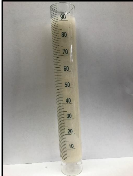
Fig. 34 – Stable proppant suspension of 40 lb/1,000 gal polymer mix 1:1 with 4 gpt crosslinker at pH 5 and 77°F for 24 hours.
