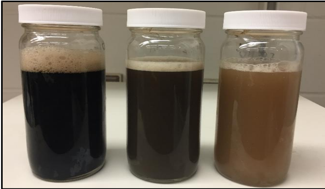
Fig. 38 – (Left) 40 lb/1,000 gal CMHPG, (Middle) 1:1 (CMHPG: Synthetic) polymer mix, (Right) Synthetic polymer, mixed with 10 ppt sodium bromate and 4 gpt crosslinker at pH 5 and 300°F for 72 hours.
