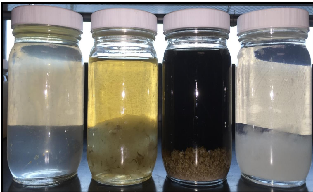
Fig. 39 – Influence of Breakers, (left to right) enzyme, chlorous acid, sodium bromate, and sodium persulfate with 40 lb/1000 gal CMHPG at 300°F for 24 hours (Almubarak et al. 2015).
