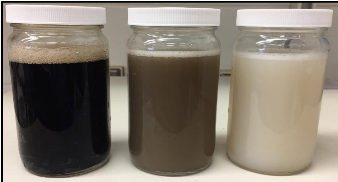
Fig. 37 – (Left) 40 lb/1,000 gal CMHPG, (Middle) 1:1 (CMHPG: Synthetic) polymer mix, (Right) Synthetic polymer, mixed with 10 ppt sodium bromate and 4 gpt crosslinker at pH 5 and 300°F for 24 hours.
