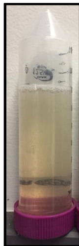
Fig. 18 – Effluent from 40 lb/1,000 gal 1:1 (CMHPG: Synthetic) polymer mixture fracturing fluid using 10 ppt bromate oxidizer at 300°F.
