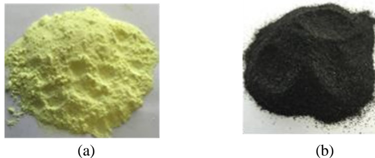
Figure 6.1 (a) Elemental Sulfur, and (b) Crumb Rubber
