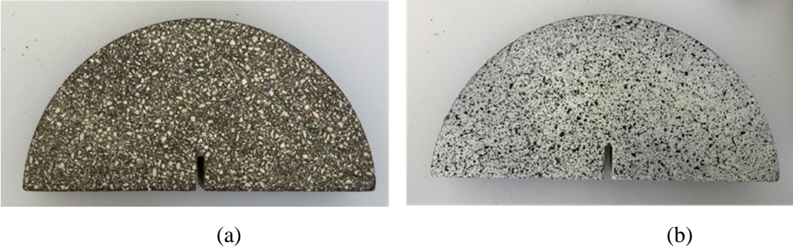
Figure 7.2 A Speckled Specimen: (a) before Painting, and (b) after Painting
