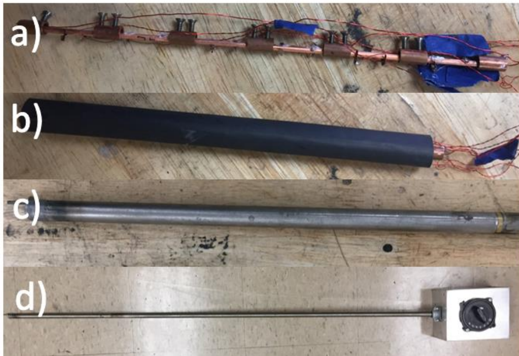
Figure 9: a) RRR couplers and samples aligned in series, b) Samples encased in heat shrink to prevent grounding to nickel-copper tube, c) 0.3m nickel-copper tube holding samples in series, d) Entire setup ready to be tested and placed in dewars
