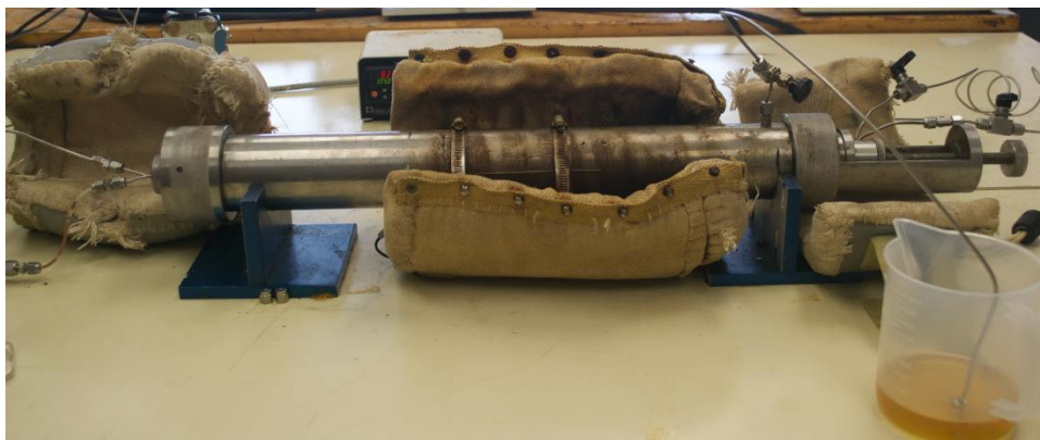
Fig. 2.17 – Hassler Type Core Holder with Heating Jackets Removed.
