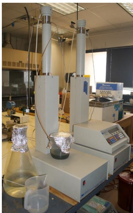
Fig. 2.15 – Syringe Pumps and Pump Controller used for Oil and Water Injection.
