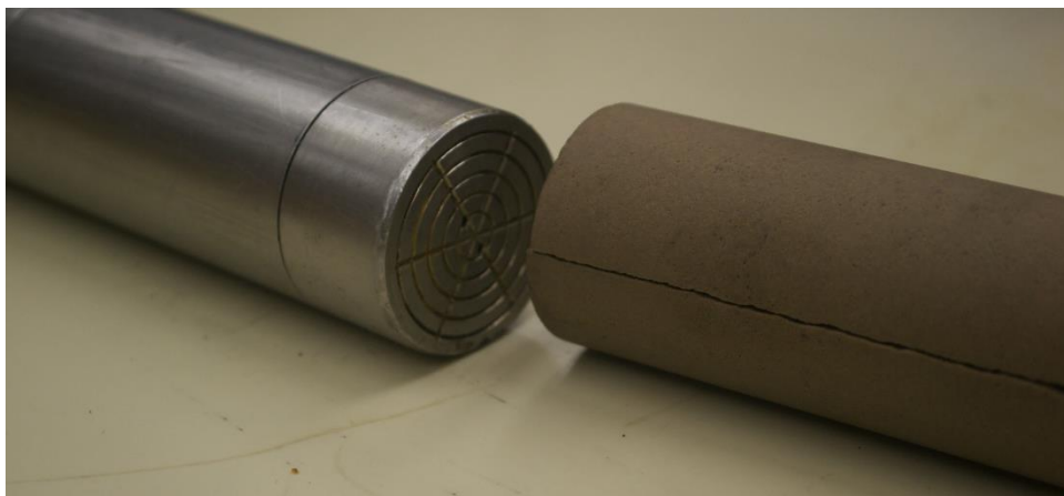
Fig. 2.20 – Close-up of Fractured Core Test Specimen and Outlet End-piece Piston Face.
