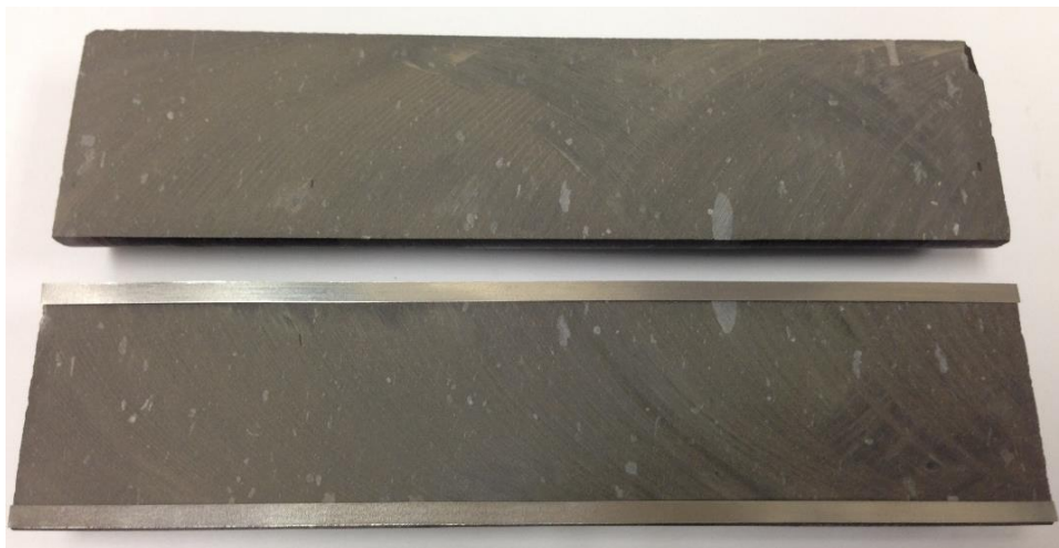
Fig. 2.8 – Example of Saw Cut Test Specimen with 100 \mu\text{m} Stainless Steel Shims to Control Fracture Aperture.
