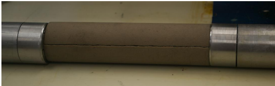
Fig. 2.19 – Close-up of Fractured Core Test Specimen in between Inlet and Outlet End-piece Pistons.
