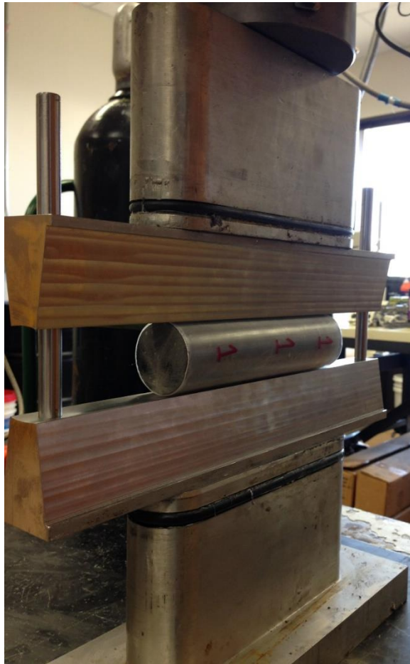
Fig. 2.4 – Test Specimen Being Fractured by Means of Indirect Tension in a GCTS Hydraulic Load Frame.
