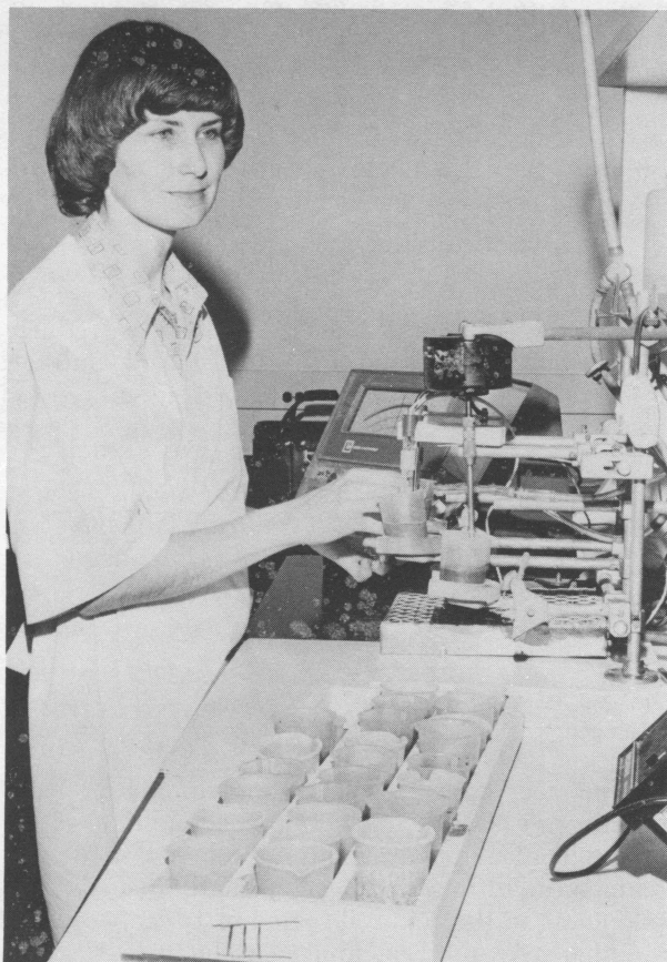
Figure 3. Soil acidity can be determined most accurately by use of the pH meter.
