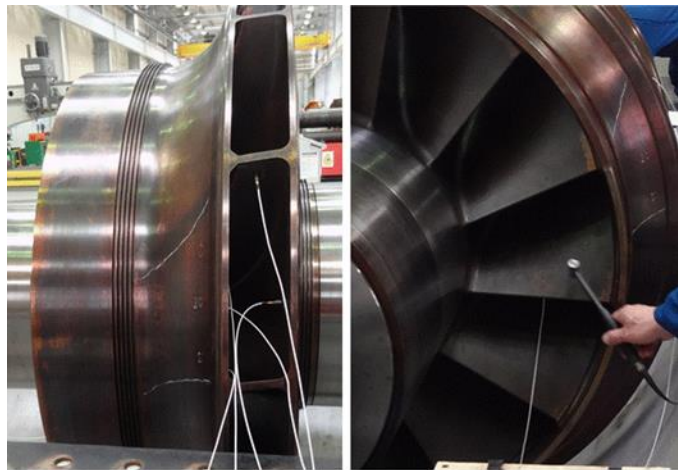
Figure 1. Photographs of Modal Testing. Impeller #1 of Propane Compressor
