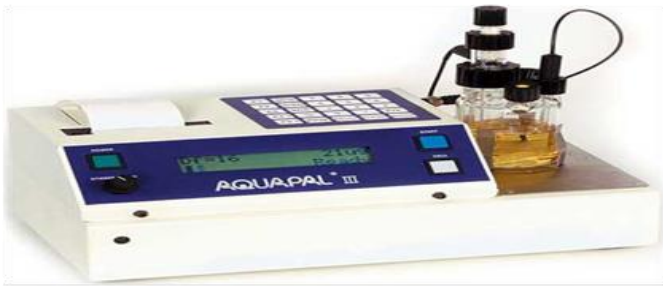
Figure 13 Measure of water content using Karl Fischer Titration method
