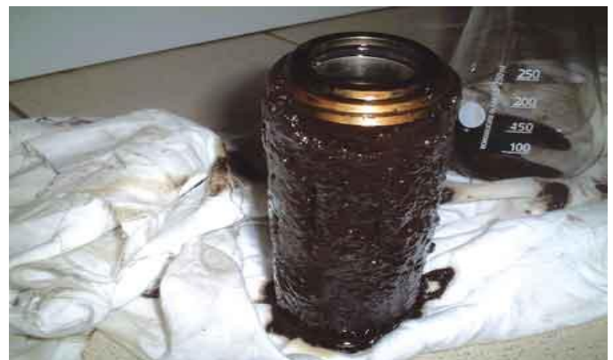
Figure 8 Severe oil oxidation resulting in plugged filters
