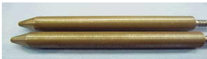
Figure 19 Lubricant without sufficient rust inhibitors
