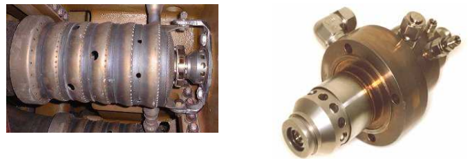
Figure 1: Conventional or Diffusion flame combustion hardware
