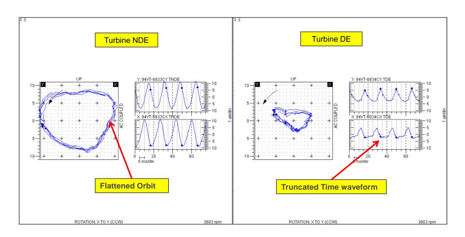
Flattened Orbit & Truncated Time Waveform due to Rub
