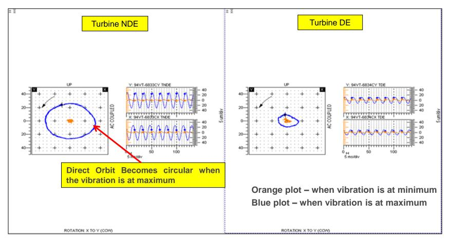
Significant change in the Orbit Shape & Amplitude
