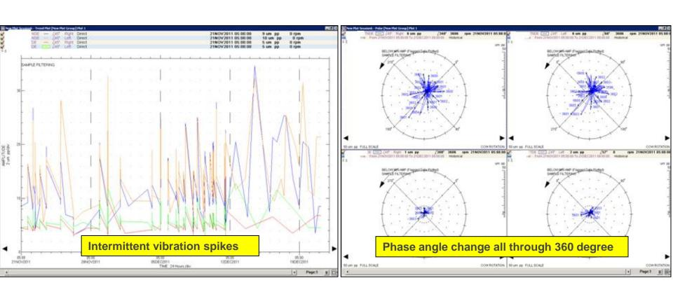
Similar Behavior But Less Severity - Intermittent vibration Amplitude & Change in Phase Angle
