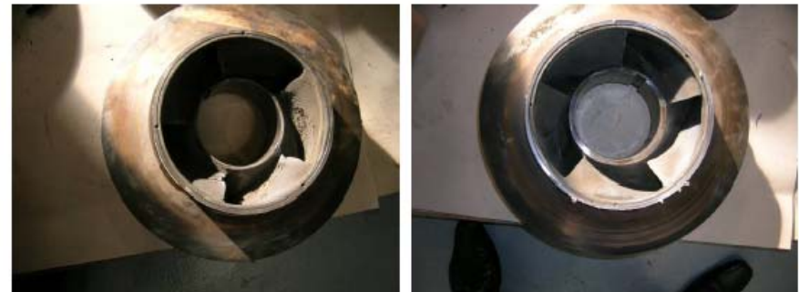
Cavitation damage on 1 st stage
