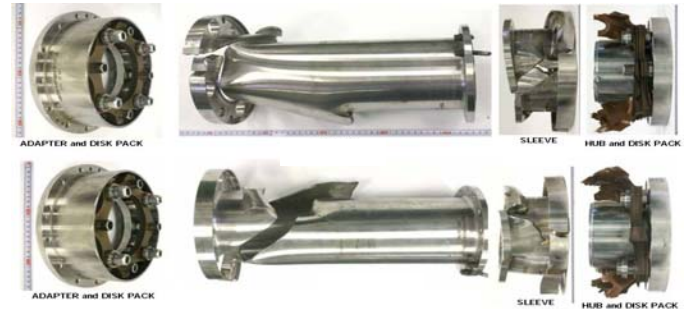
Figure 2) Spiral Failure of Spacer - Typical of Excessive Torsional Stress
