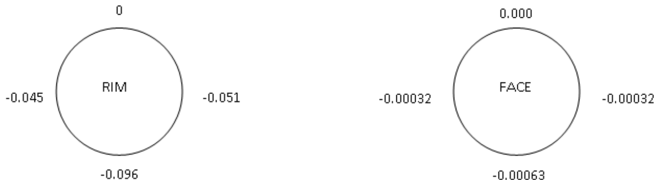
Load Gear Box to Turbine Findings After Correction (All Dimensions are in inches)
