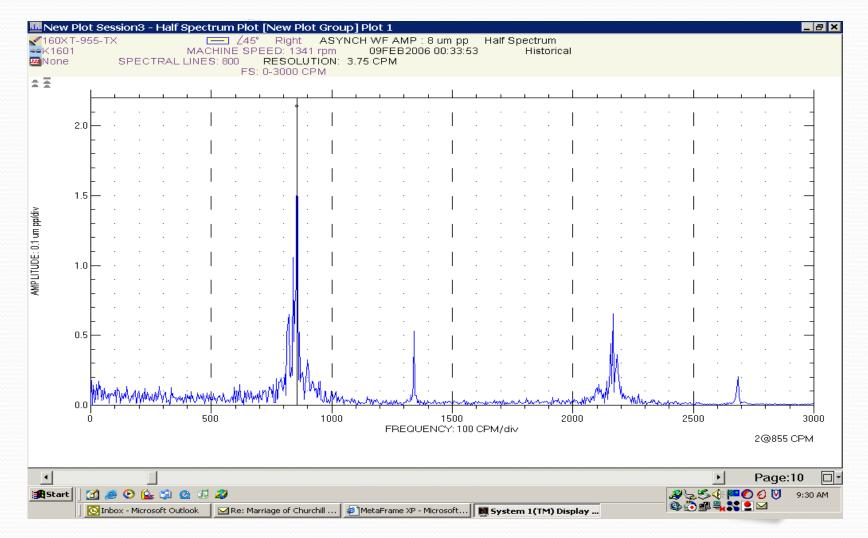
Vibration spectrum on bull gear after tuning the VSD
