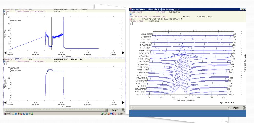
Overall vibration plot with speed and coast down waterfall from hard stop
