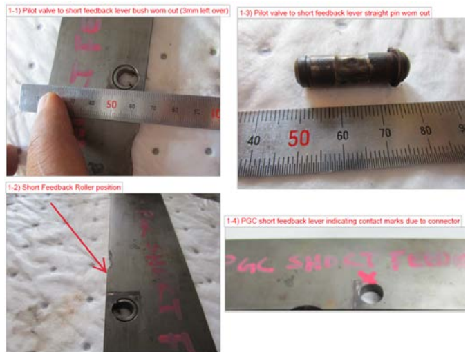
Figure 6: Lever and deva-metal wear
