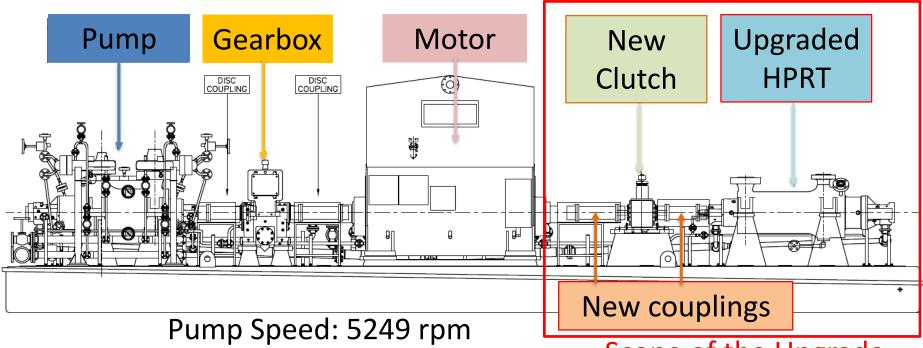
Motor/ HPRT Speed: 2980 rpm
