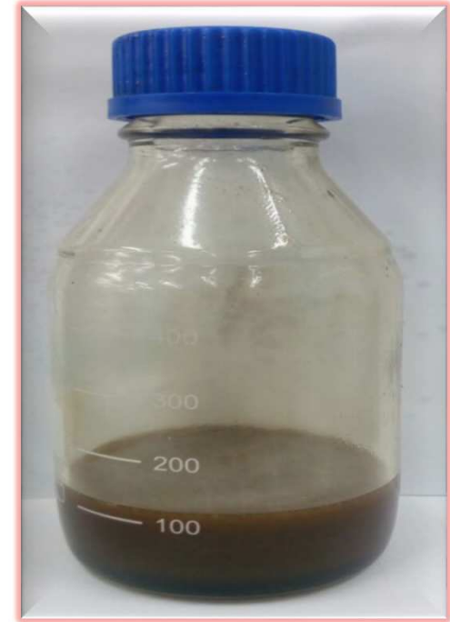
Carried-over Lube @ GTG Fuel Gas Filter
