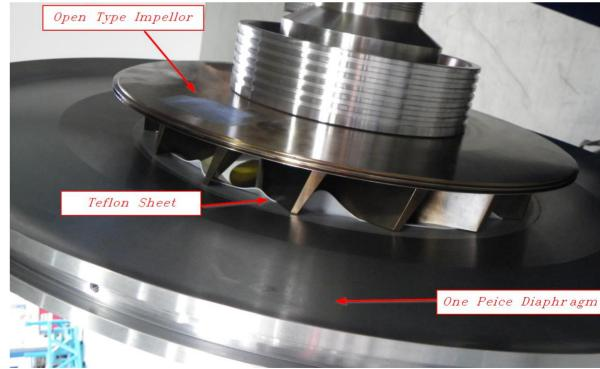
A trial assembly of the tooling to lock the shaft/impeller assembly to the one piece diaphragm was performed
