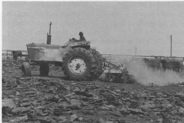
Figure 3. Chisel plowing the manure pack prior to collection with a wheel loader increases productivity and reduces energy consumption by at least one-third.
