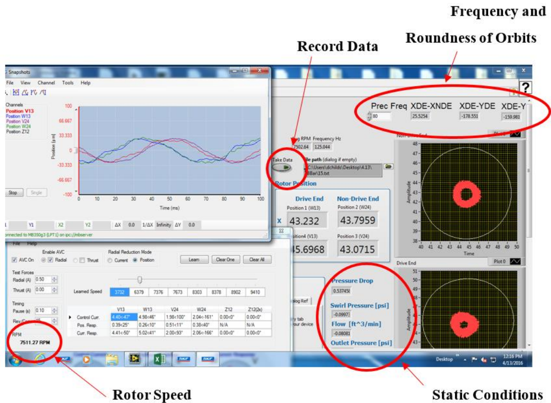
Figure 29. Monitoring tools and Input VI used while testing at 7.5 kRPM.
