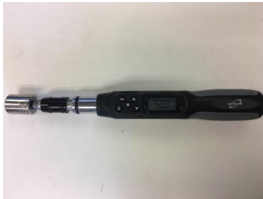
Figure 9. Photograph of digital torque screwdriver. (Range : 50-500 N-mm, Resolution : 1 N-mm, Accuracy : \pm 2\% of CW, \pm 3\% of CCW)
