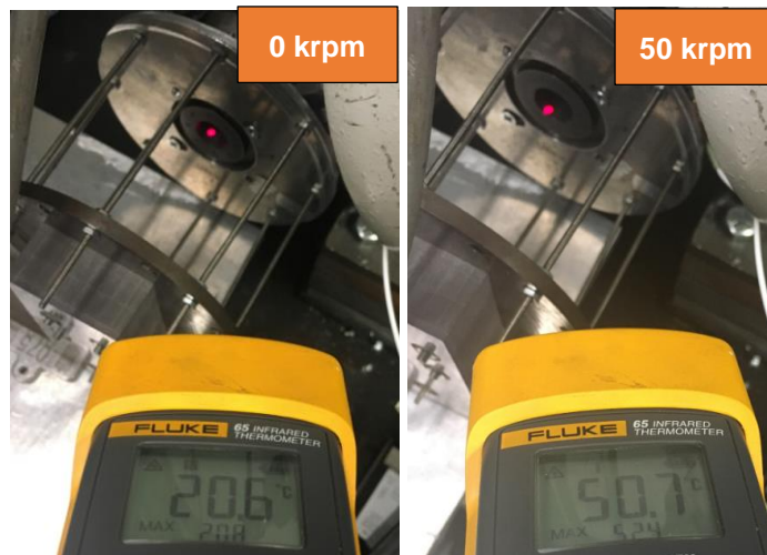
Figure 33. Photographs of bearing cartridge and shaft – measurement of temperature. (left : 0 krpm, \sim 20.6^{\circ}\text{C} , right : at 50 krpm, \sim 50.7^{\circ}\text{C} )
