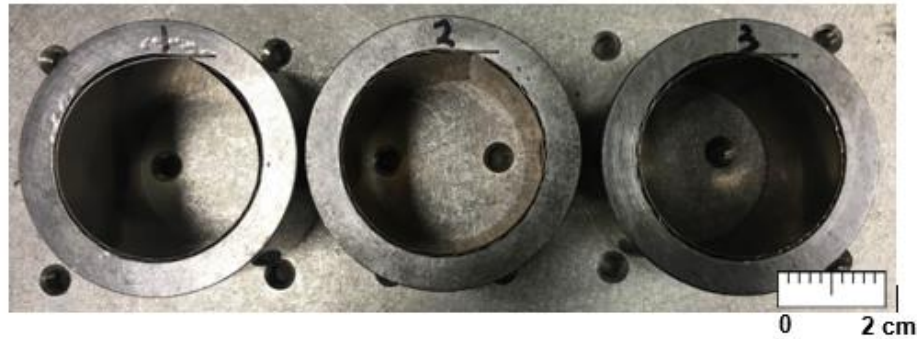
Figure 3. Photograph of test bearings (Left : Uncoated, Center : TiSiN, Right : VN).
