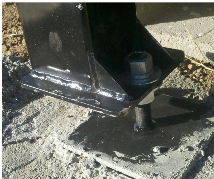
Figure 15. Adjustable screw used to adjust the angle of the IR source trailer.
