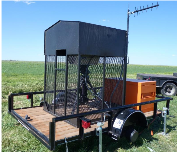
Figure 12. Spectrometer mounted on a trailer and protected by a cage enclosure.
