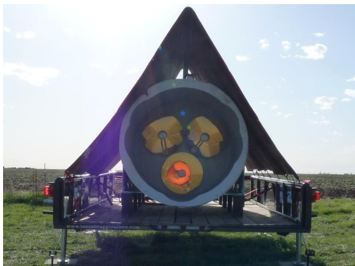
Figure 11. IR source mounted on a trailer and supported by four trailer jacks.
