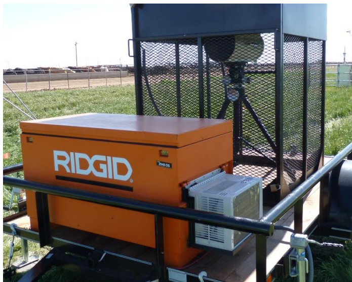
Figure 16. Weather sealed box containing computer and supplemental equipment.
