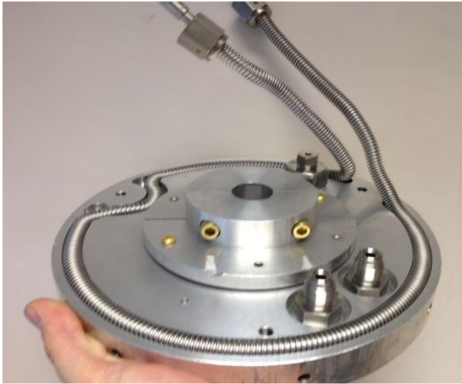
Figure 22. Outer shield support attached to EM clamp
