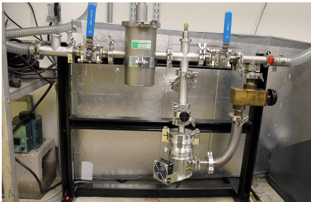
Figure 31. The high vacuum system (mechanical pump not shown)
