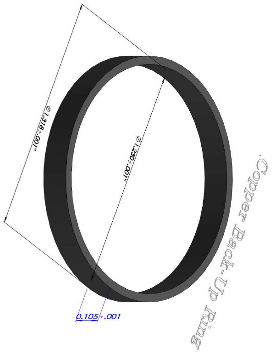
Figure A.2 Copper back-up ring drawing with dimensions
