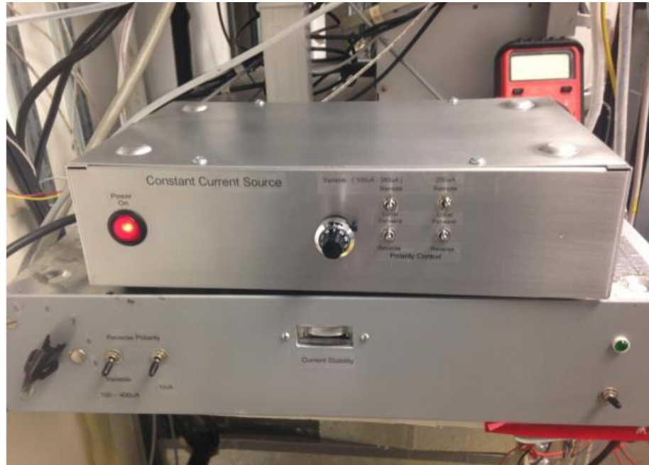
Figure 32. Current sources fabricated by the physics electronics shop at TAMU
