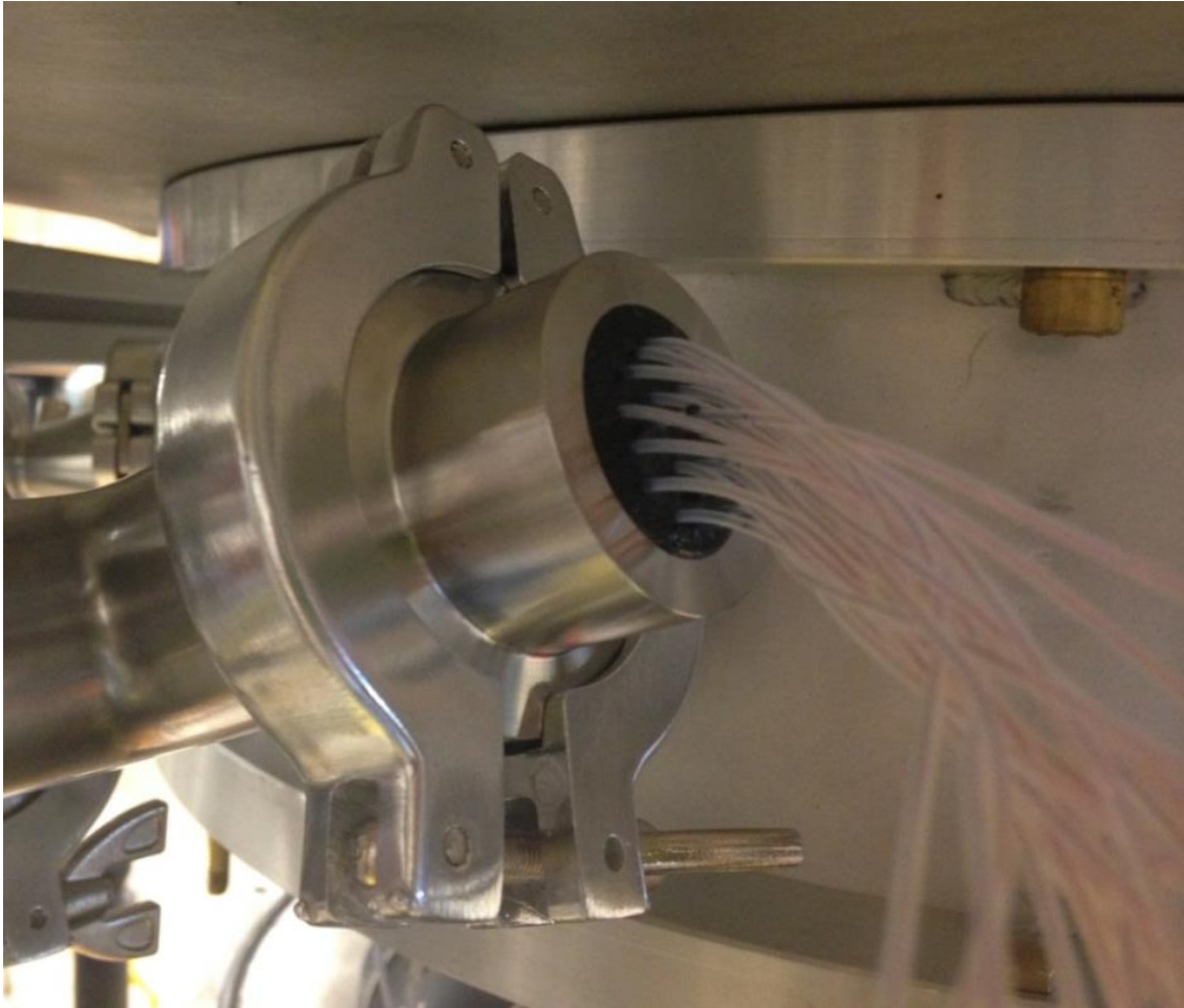
Figure 27. RTD feedthrough flange
