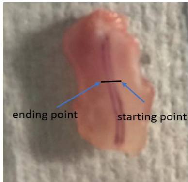
Figure 6. Starting and ending point of line scan. Data was acquired every 50 or 100 \mu\text{m} .
