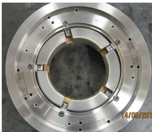
Figure 14 – Integral squeeze film damper installed on the CCTV.
