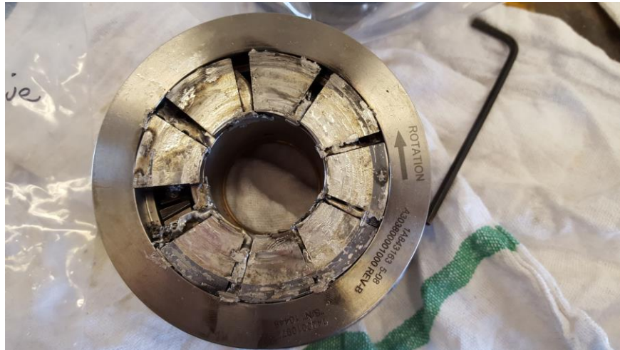
Figure 15: Pinion 2 Inactive Thrust Bearing Damage
