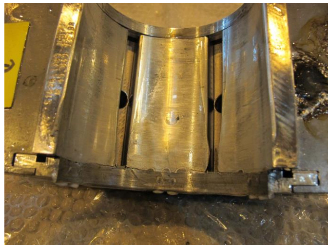
Figure 3: Damaged Pinion Bearing
