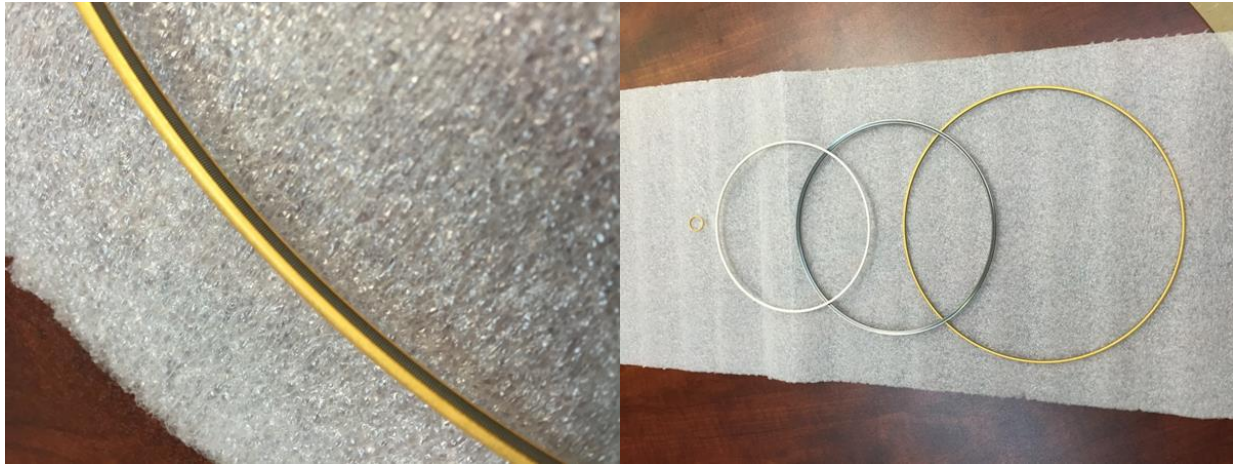
Figure 13. Metallic C-Seals for High Temperature
