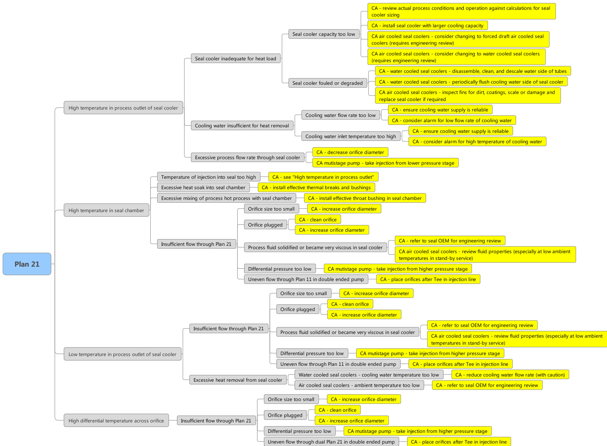
Figure 18 RCA Piping Plan 21
