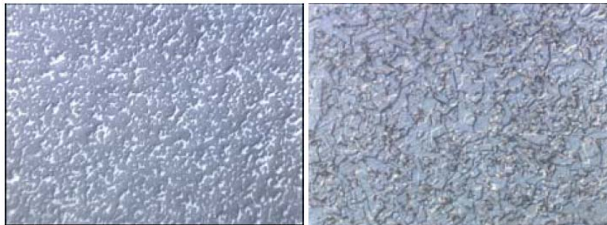
Figure 6: Reaction bonded (left) and sintered (right) silicon carbide surfaces
