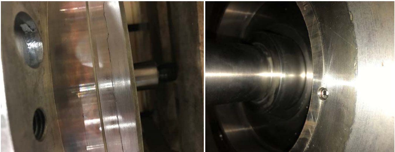
Figure 3: Monel overlay on pump head fit (left) and wear ring area (right)
