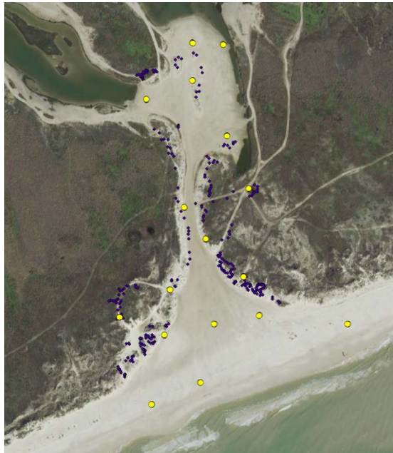
Figure 7. Locations of GCPs (yellow) and VPs (purple). Note: each yellow dot in the figure consist of two GCPs.
