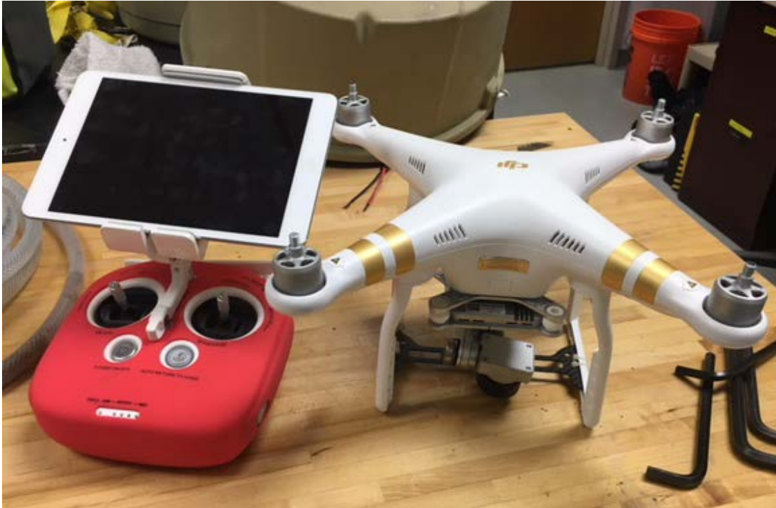
Figure 2. DJI Phantom 3 Professional with detachable propellers (not pictured).
