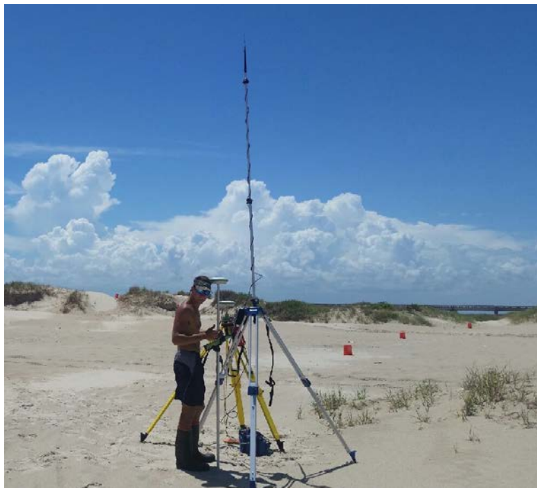
Figure 3. RTK-GPS deployed for test flights at San Luis Pass, Texas.
