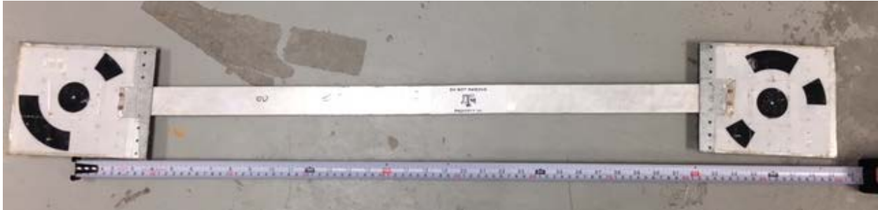
Figure 4. Ground control marker bar with two markers, 3 feet apart.
