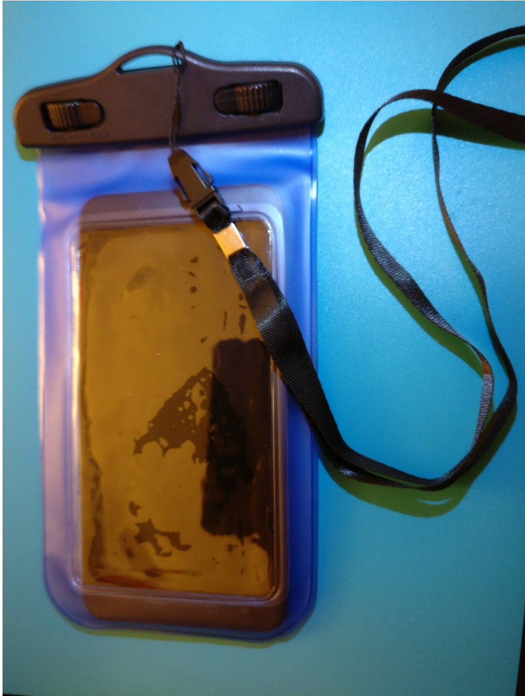
Figure 4.2: Smartphone inside the small waterproof pouch used for when testing the recognition algorithm.
