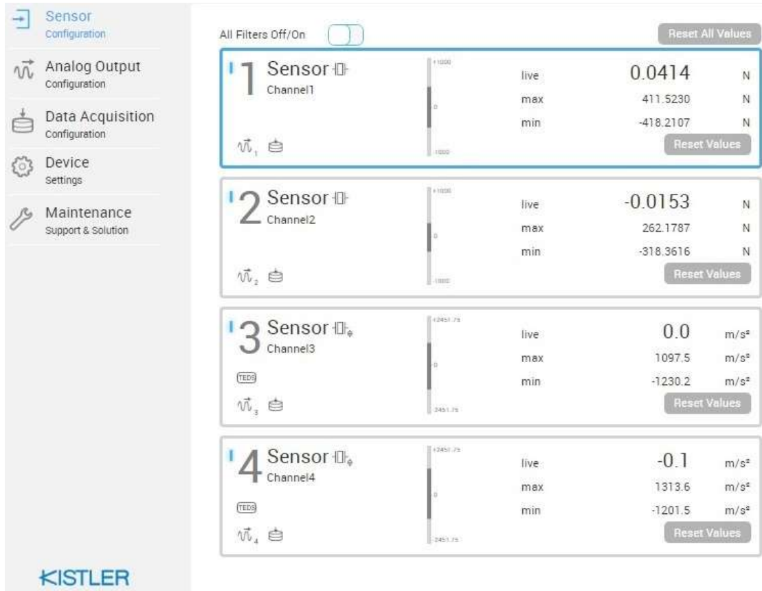
Figure 17: Kistler Lab amplifier interface: takes voltages from the accelerometer and dynamometer and outputs that data to be run through a MATLAB code. Sensors 1 and 2 are the thrust force and cutting force respectively, while sensors 3 and 4 are the thrust acceleration and cutting acceleration respectively
