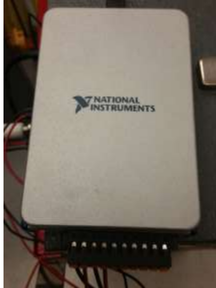
Figure 14: National Instruments Data Acquisition System: takes voltage signals from the signal amplifier and sends them to a LabVIEW program for processing. The model used was a NI-9215 DAQ coupled with a cDAQ-9171 Chassis.
