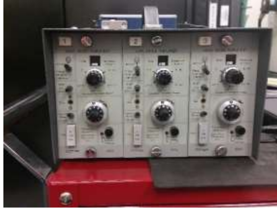
Figure 12: The signal amplifier takes the small voltages given off by the dynamometer, amplifies them, and then feeds them into the DAQ
