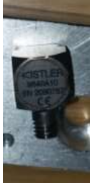
Figure 11: The accelerometer measures changes in velocity, and converts them into an electrical signal for the DAQ to read
