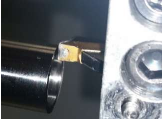
Figure 6: The tool insert used had a width greater than the width of the workpiece, therefore only two forces were induced. Thrust and cutting forces are present, as feed direction and depth of cut direction are the same.
