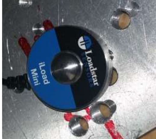
Figure 21: Loadstar iLoad Mini load cell used in calibration. (See specifications below)
