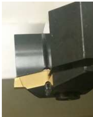
Figure 19: Coated Tungsten Carbide-Cobalt Grooving Tool
