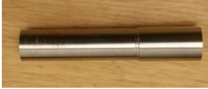
Figure 18: Ti-6Al-4V Tube OD = 0.645", ID = 0.0484"
