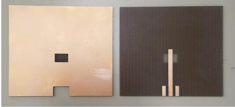
Figure 13. Ground plane with slot (left) and microstrip plane (right)
