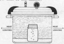
7. If the vent is opened before the pressure reaches zero or too soon after pressure falls to zero, there is danger of jars exploding. This sudden release of outside pressure permits steam to form explosively in the jar and the liquid boils out.
