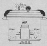
2. As heating continues, air is finally exhausted. Air must be excluded because it interferes with passage of heat. Heat passes through steam more readily than through air. Heat continues to penetrate the jar.
