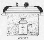
6. At the end of the processing time, the source of heat is removed and active boiling stops. Temperature and pressure in the canner start to fall as the cooling-off period begins. Temperature and pressure in the jar slowly follow that of the canner.
