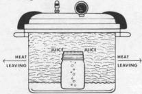
3. When the canner is removed from heat and the petcock is left closed, cooling continues slowly. The gauge needle returns to zero. The vent is opened slowly. Air enters from
