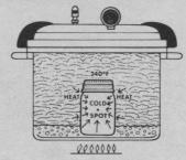
B. Heat is also distributed by convection. Heated fluids expand, rise and are replaced by cooler fluids. Convection currents are slow in thick mixtures. They are retarded by fat, tightly-packed food and solid materials. Heat penetrates by both convection and conduction at the same time.
