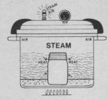
3. The vent is closed after steam has escaped for 10 minutes. Steam now cannot escape, so pressure rises. Water under pressure boils at temperatures above 212° F. At 5 pounds gauge pressure, water boils at 228° F. At 10 pounds pressure, water boils at 240° F.
