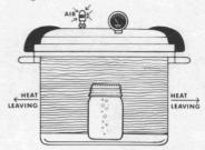
9. After jars are removed from the canner, the contents may continue to boil as the jar pressure is reduced by condensation of steam. Continued boiling is a good indication that jars are tightly sealed.
